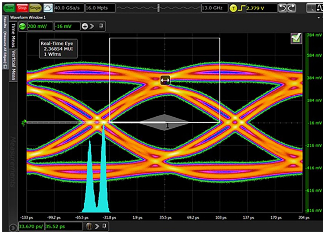
Fig. 11. HDMI 2.1 6 Gbps TMDS eye diagram, PCB with device; typical values
