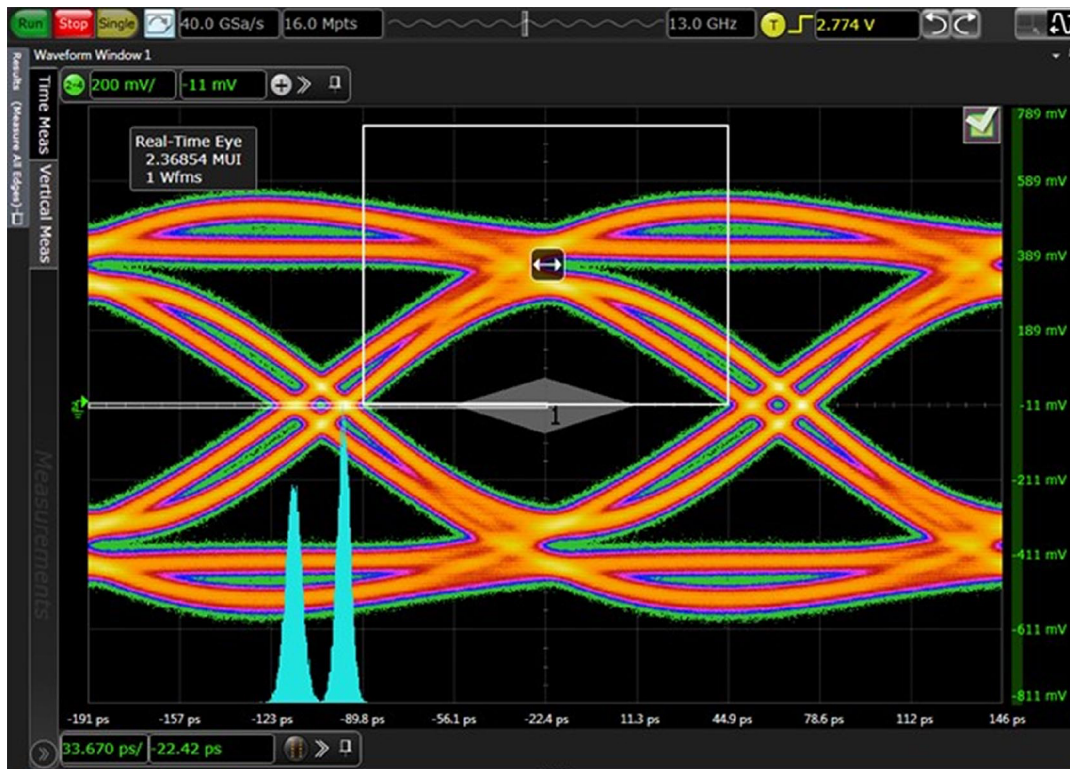
Fig. 11. HDMI 2.1 6 Gbps TMDS eye diagram, PCB with device; typical values
