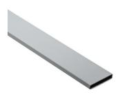
A temporary film is applied to the covers to protect against scratches and is writable for identification during installation. Cover is flush with the side of the duct for increased wire capacity and allows for tight, side-by-side duct placement.
