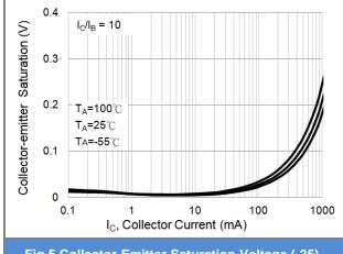
Fig.5 Collector-Emitter Saturation Voltage (-25)
