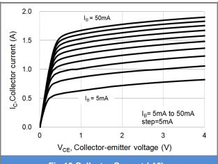
Fig.10 Collector Current (-16)
