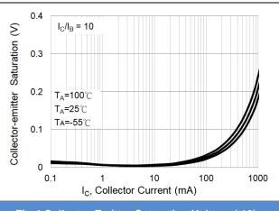
Fig.4 Collector-Emitter Saturation Voltage (-16)
