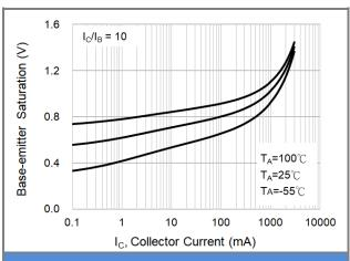
Fig.9 Base-Emitter Saturation Voltage (-40)
