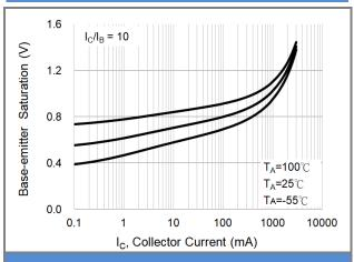
Fig.7 Base-Emitter Saturation Voltage (-16)
