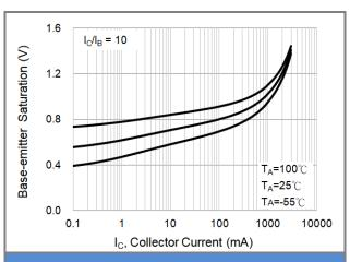
Fig.8 Base-Emitter Saturation Voltage (-25)
