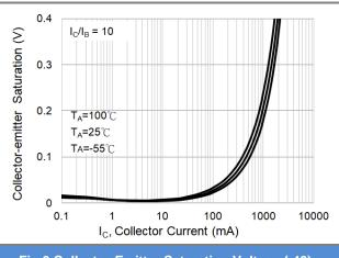
Fig.6 Collector-Emitter Saturation Voltage (-40)
