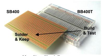
Move Your Circuit From a BB400 Solderless Plug-in BreadBoard To a Permanent Solderable PC BreadBoard
