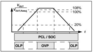
Figure 7 V<sub>OUT</sub> Related Protection Features
