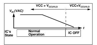
Figure 6 V<sub>IN</sub> Related Protection Features
