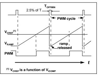
Figure 13 Ramp and PWM waveforms
