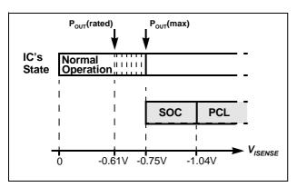
Figure 8 SOC and PCL Protection as function of V<sub>ISENSE</sub>
