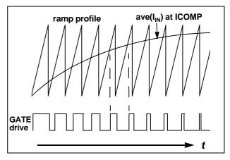
Figure 12 Average Current Control in CCM
