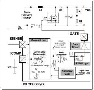
Figure 11 Complete System Current Loop
