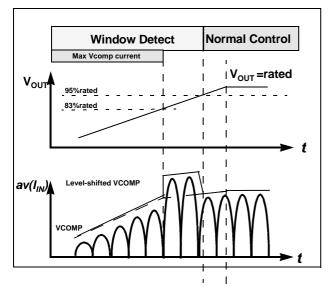
Figure 5 Startup with controlled maximum current
