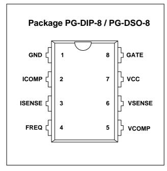
Figure 1 Pin Configuration (top view)
