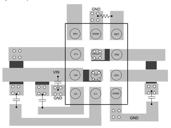
Figure 16. LM2758 Layout Example
