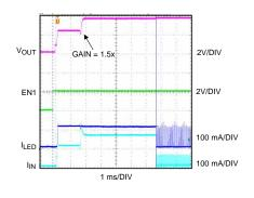
$V_{IN} = 3.6 \text{ V}$   $I_{LED} \text{ (torch)} = 108 \text{ mA}$  EN2 = 0 V
