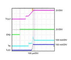
$V_{IN} = 3.6 \text{ V}$ EN1 = 0 V  $I_{LED} = 108 \text{ mA}$
