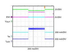
$EN2 = V_{IN} = 3.6 \text{ V}$   $I_{LED} \text{ (flash)} = 500 \text{ mA}$
