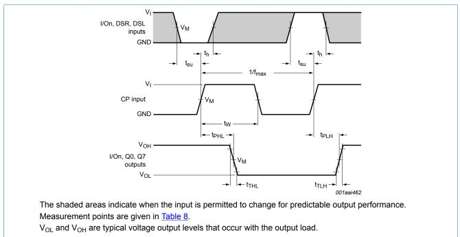
Fig. 6. Clock pulse to outputs I/On, Q0, Q7 propagation delays, the clock pulse width, the I/On, DSR and DSL to clock pulse set-up and hold times, the output transition times and the maximum clock frequency
