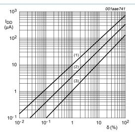
$R_{EXT}$  = 100 kΩ;  $C_{EXT}$  = 100 nF;  $C_L$  = 50 pF; one monostable multivibrator switching only
