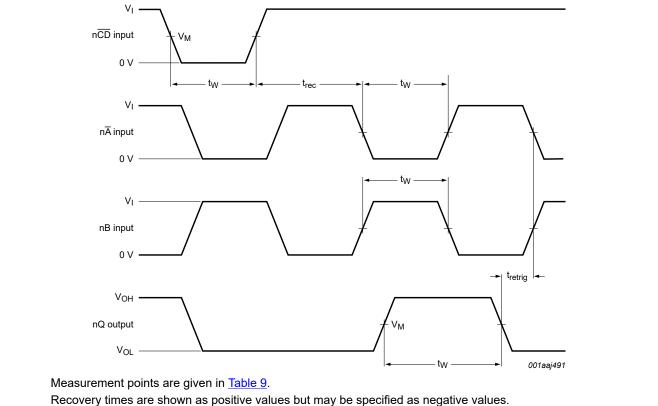
Logic levels: V<sub>OL</sub> and V<sub>OH</sub> are typical output levels that occur with the output load.
