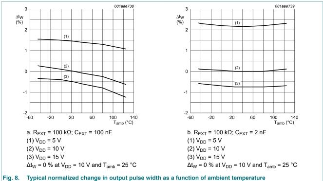
Typical normalized change in output pulse width as a function of ambient temperature
