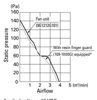
Applied voltage: 12 VDC \* Finger guard is attached on air inlet side of fan.
