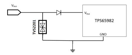
Figure 7. TVS2201 Application Schematic
