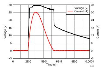
Figure 8. TVS2201 Surge Clamping at 30 A
