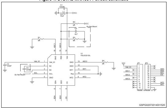
Figure 1. STEVAL-MKI153V1 circuit schematic
