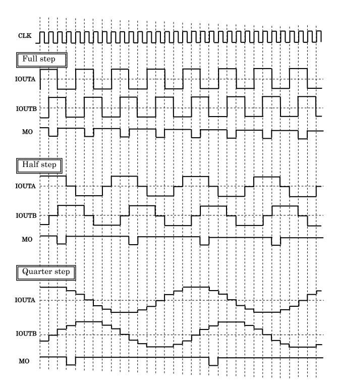
The MO is an open drain output pin. Therefore the High level of the MO waveform shown above, will be the MO pin's pulled up voltage level.
