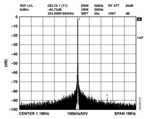
Figure 10. NBSFDR,  $\pm 1$  MHz,  $f_{OUT} = 1.1$  MHz,  $f_{CLK} = 500$  MSPS
