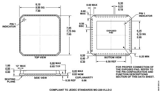
Figure 50. 56-Lead Lead Frame Chip Scale Package [LFCSP\_VQ] 8 mm × 8 mm Body, Very Thin Quad (CP-56-1) Dimensions shown in millimeters
