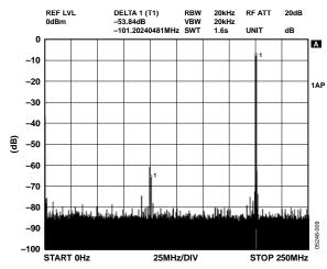
Figure 9. Wideband SFDR,  $f_{OUT} = 200.3 \text{ MHz}$ ,  $f_{CLK} = 500 \text{ MSPS}$
