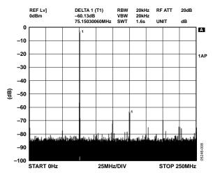
Figure 8. Wideband SFDR,  $f_{OUT} = 75.1$  MHz,  $f_{CLK} = 500$  MSPS
