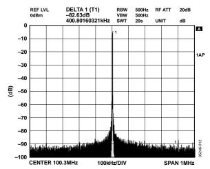
Figure 12. NBSFDR,  $\pm 1$  MHz,  $f_{OUT} = 100.3$  MHz,  $f_{CLK} = 500$  MSPS
