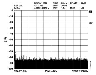
Figure 4. Wideband SFDR,  $f_{OUT} = 1.1$  MHz,  $f_{CLK} = 500$  MSPS
