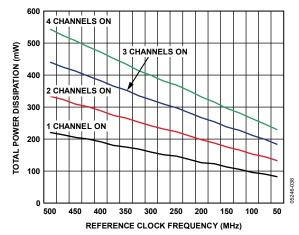
Figure 20. Power Dissipation vs. Reference Clock Frequency vs. Channel(s)
