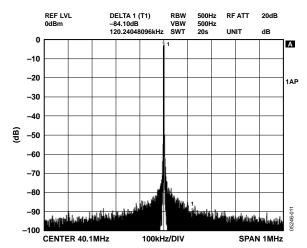
Figure 11. NBSFDR,  $\pm 1$  MHz,  $f_{OUT} = 40.1$  MHz,  $f_{CLK} = 500$  MSPS
