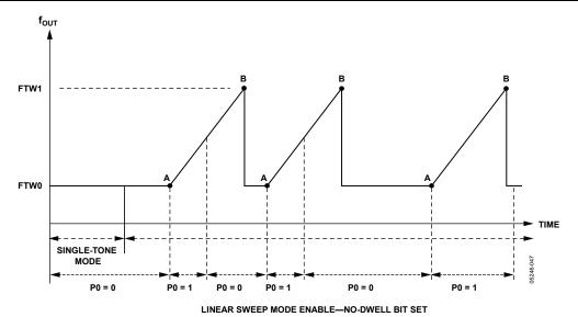
Figure 38. Linear Sweep Mode (No-Dwell Enabled)
