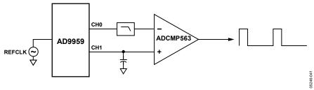
Figure 27. Agile Clock Source with Duty Cycle Control Using the Phase Offset Value in DDS to Change the DC Voltage to the Comparator
