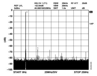
Figure 5. Wideband SFDR,  $f_{OUT} = 40.1 \text{ MHz}$ ,  $f_{CLK} = 500 \text{ MSPS}$
