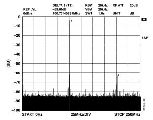
Figure 6. Wideband SFDR,  $f_{OUT} = 100.3 \text{ MHz}$ ,  $f_{CLK} = 500 \text{ MSPS}$
