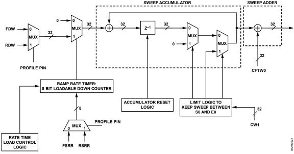
Figure 37. Linear Sweep Block Diagram (Frequency Sweep)
