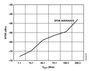
Figure 21. Averaged Channel SFDR vs. four
