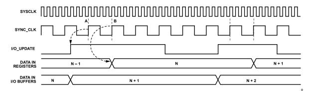
THE DEVICE REGISTERS AN I/O UPDATE AT POINT A. THE DATA IS TRANSFERRED FROM THE ASYNCHRONOUSLY LOADED I/O BUFFERS AT POINT B. Figure 40. I/O\_UPDATE Transferring Data from I/O Buffer to Active Registers
