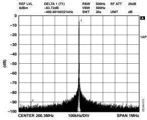
Figure 15. NBSFDR,  $\pm 1$  MHz,  $f_{OUT} = 200$ . 3MHz,  $f_{CLK} = 500$  MSPS
