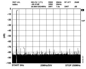
Figure 7. Wideband SFDR,  $f_{OUT} = 15.1 \text{ MHz}$ ,  $f_{CLK} = 500 \text{ MSPS}$
