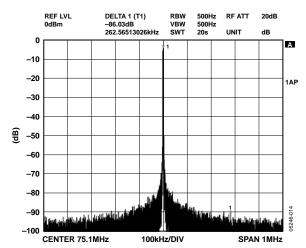
Figure 14. NBSFDR,  $\pm 1$  MHz,  $f_{OUT} = 75.1$  MHz,  $f_{CLK} = 500$  MSPS
