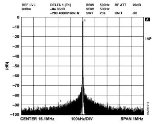
Figure 13. NBSFDR,  $\pm 1$  MHz,  $f_{OUT} = 15.1$  MHz,  $f_{CLK} = 500$  MSPS
