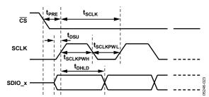
Figure 41. Setup and Hold Timing for the Serial I/O Port
