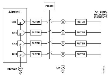
Figure 22. Phase Array Radar Using Precision Frequency/Phase Control from DDS in FMCW or Pulsed Radar Applications;
