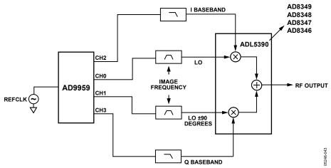
Figure 23. Single-Sideband-Suppressed Carrier Upconversion
