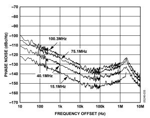
Figure 17. Residual Phase Noise (SSB) with  $f_{OUT}$  = 15.1 MHz, 40.1 MHz, 75.1 MHz, 100.3 MHz;  $f_{CLK}$  = 500 MHz with REFCLK Multiplier = 5×
