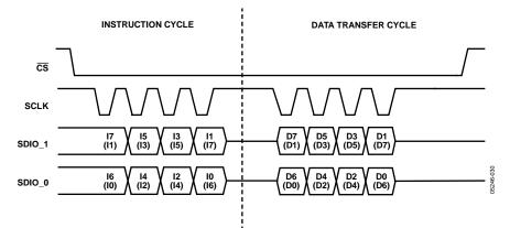
Figure 48. 2-Bit Serial Mode Read Timing—Clock Stall High
