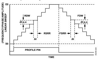
Figure 36. Linear Sweep Parameters
