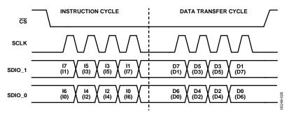
Figure 44. 2-Bit Serial Mode Write Timing—Clock Stall Low
