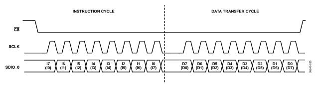
Figure 43. Single-Bit Serial Mode Write Timing—Clock Stall Low
