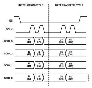
Figure 45. 4-Bit Serial Mode Write Timing—Clock Stall Low
