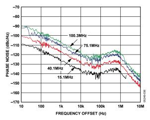
Figure 18. Residual Phase Noise (SSB) with  $f_{OUT}$  = 15.1 MHz, 40.1 MHz, 75.1 MHz, 100.3 MHz;  $f_{CLK}$  = 500 MHz with REFCLK Multiplier = 20×
