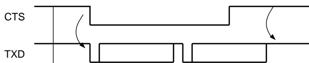
Figure 31-21. Transmitter Behavior when Operating with Hardware Handshaking
