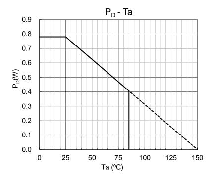
When mounted on a single-side glass epoxy board (50 mm × 50 mm × 1.6 mm, Cu area: 40%, Cu thick: 35 µm)
