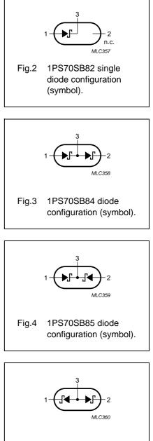
Fig.5 1PS70SB86 diode configuration (symbol).
