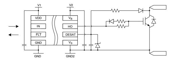
Figure 2. Simplified Application Schematics
