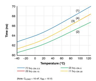
Figure 29. High Propagation Delay
