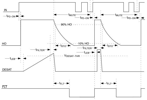
Figure 6. DESAT Response Waveform
