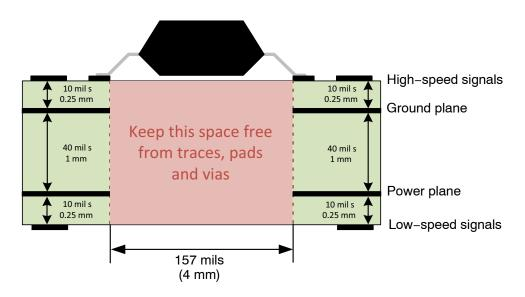
Figure 41. Recommended Layer Stack
