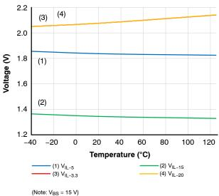
Figure 16. Low Input Voltage
