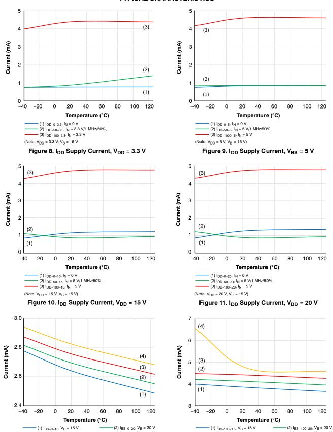
Figure 12. I<sub>BS</sub> Supply Current, V<sub>DD</sub> = 5 V
