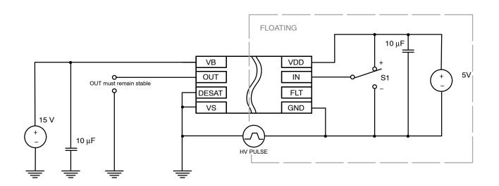
(Test Conditions: HV Pulse  $\pm 1500$  V, dV/dt = 1–100 V/ns,  $V_{DD}$  = 5 V,  $V_{BS}$  = 15 V)
