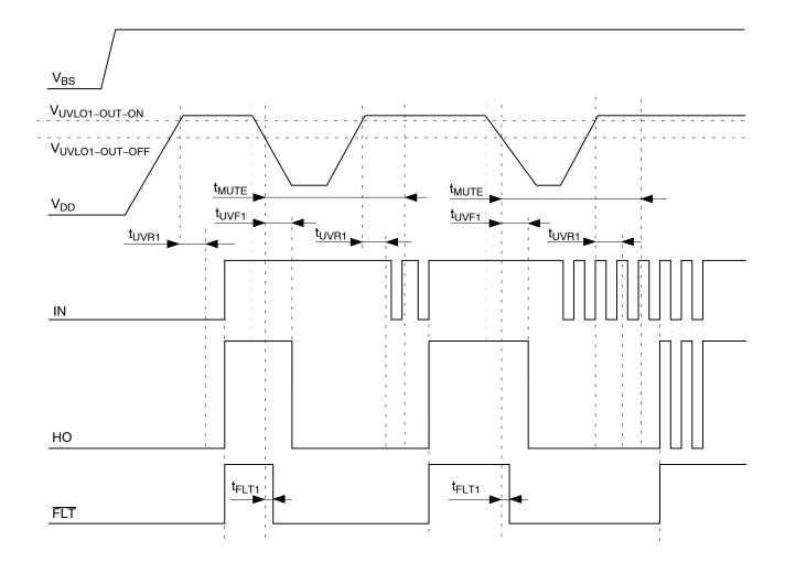
Figure 4. UVLO1 Waveform
