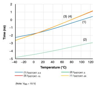
Figure 31. Propagation Delay Distortion
