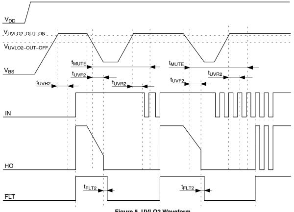
Figure 5. UVLO2 Waveform
