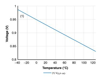
Figure 28. IGBT Short Circuit Clamping Voltage
