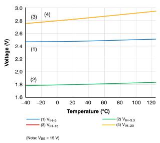
Figure 17. High Input Voltage
