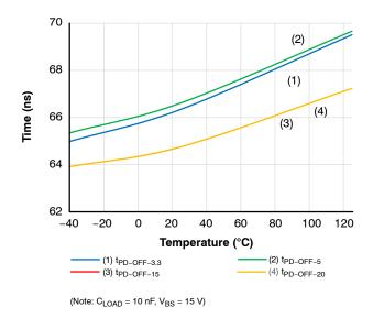
Figure 30. Low Propagation Delay
