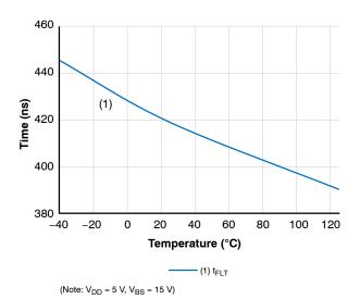
Figure 35. FLT Delay Time
