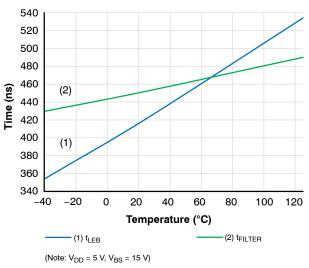
Figure 33. DESAT Threshold Filtering Time, DESAT Leading Edge Blanking Time
