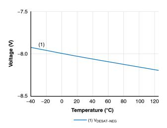
Figure 24. DESAT Threshold Voltage
