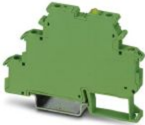
Input solid-state relay terminal block, input: 5 V DC, output: 3 - 48 V DC/100 mA, terminal block width: 6.2 mm
