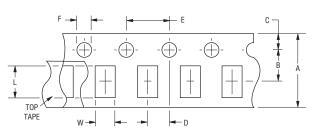
NOTES: TAPE MATERIAL IS PAPER. TAPE THICKNESS IS:  $\frac{0.6\pm0.03}{(0.024\pm0.0012)}$  COVER TAPE ADHESION IS 35  $\pm25$  GRAMS.
