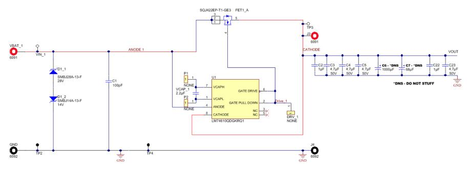
Figure 9. LM74610-SQEVM Schematic
