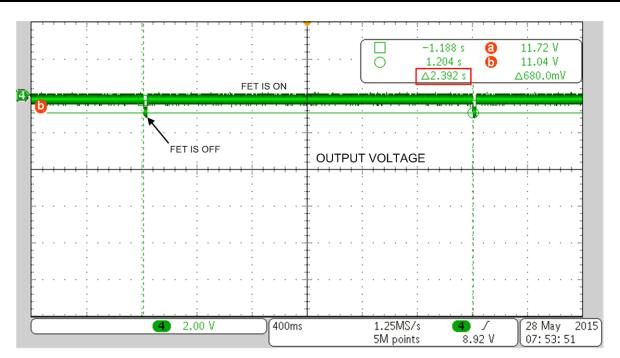
Figure 6. The LM74610-SQEVM Output voltage waveform
