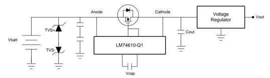
Figure 1. LM74610-Q1 Typical Application Circuit
