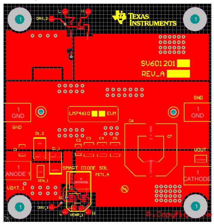
Figure 7. Top Assembly Layer
