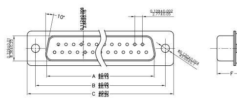
Material & Finish Shell: Steel Nickel or Tin plated
