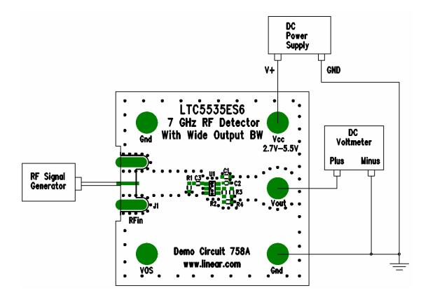
Figure 1. Proper Measurement Equipment Setup
