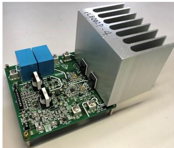
Figure 21. Heatsink Installation Example
