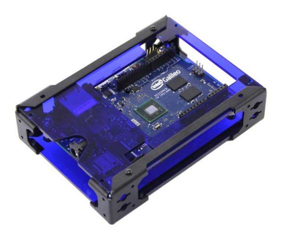
When you have a Galileo PCB, do you want to select a suitable case for improving whole felling and protecting it? There is a case that we customize for the PCB. The Case is used to wrap the Galileo PCB, It's constructed from military grade alminum and hardwearing acrylic, Providing the ultimate protection from physical and corrosion!Because we use blue acrylic, So it looks very neatly and beautiful
