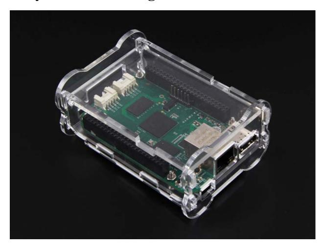
The enclosure provides slots to access the Grove, USB ports, Ethernet, SD card, HMDI, and JTAG connectors as well as feet and vents to ensure the board gets proper cooling. All of the status LEDs on the board are visible through the case thanks to light pipes embedded in the design. This is a really slick case and once you've gotten your hands on BeagleBone Green, you'll want to snag one of these to put it in!
