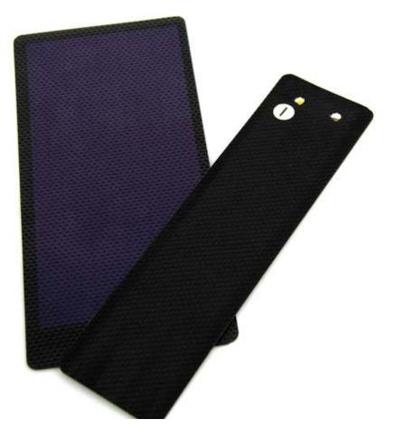
The Thin-film flexible solar panel is built on an ultra-thin backsheet. It can be installed in a curve of up to 30 degrees. In addition to its unique flexibility. It packaging with durable, high light transmittance ETFE film and fast curing EVA film.
