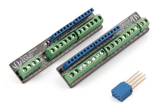
Screw shield is a wing-like shield that extends both sides of your Arduino or Arduino variants into sturdy and reliable screw terminal blocks.
