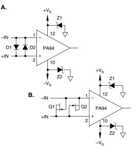
Conditions which can cause open circuits or polarity reversals on either power supply rail should be avoided or protected against. Reversals or opens on the negative supply rail is known to induce input stage failure. Unidirectional transzorbs prevent this, and it is desirable that they be both electrically and physically as close to the amplifier as possible.
