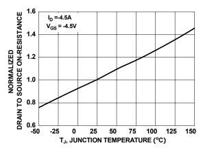
Figure 3. Normalized On-Resistance vs Junction Temperature
