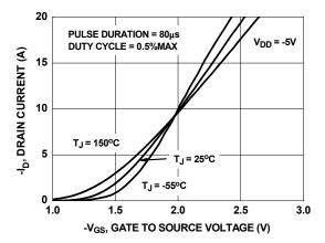
Figure 5. Transfer Characteristics
