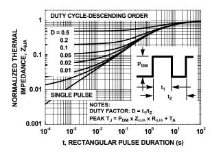
Figure 12. Transient Thermal Response Curve
