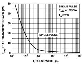
Figure 11. Single Pulse Maximum Power Dissipation
