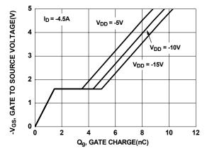
Figure 7. Gate Charge Characteristics
