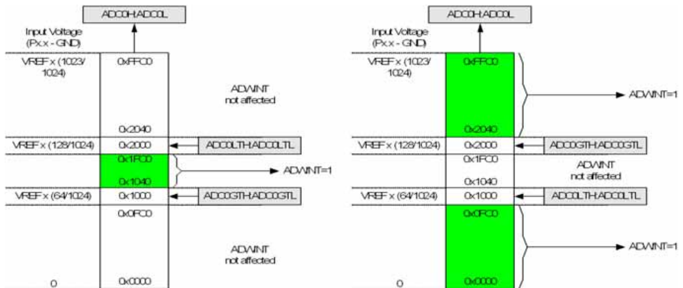
Figure 14.7. ADC Window Compare Example: Left-Justified Single-Ended Data
