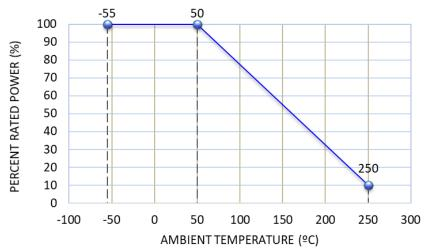
Note: This curve assumes the part is mounted on a properly sized heat sink.
