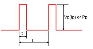
Where: Vp: Pulse limiting voltage (V)
