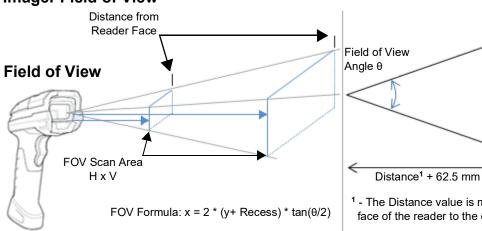
Note: The Recess value of 62.5 mm is the distance from the reader front face to the image sensor inside the reader. The Distance and Recess values are added together for the FOV Scan Area calculation.
