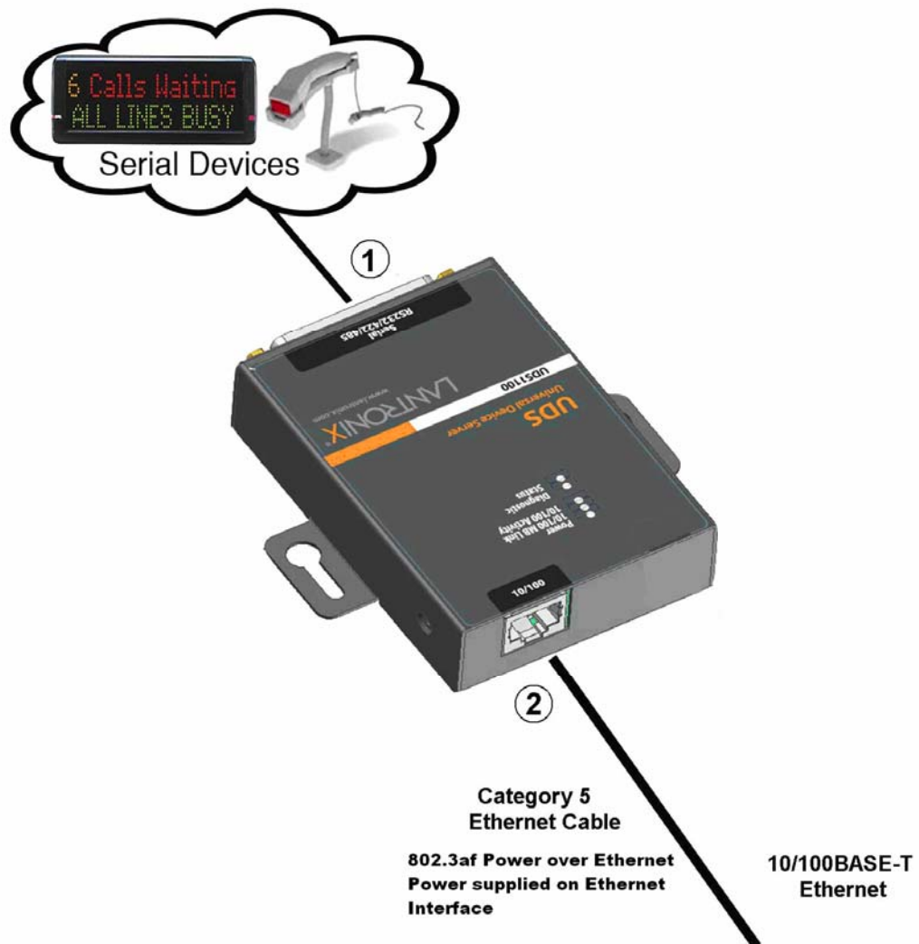
Figure 3-1. UDS1100-POE Version Connected to Serial Device and Network
