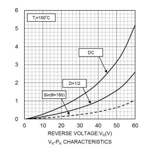
REVERSE POWER DISSIPATION:P<sub>R</sub>(mW)
