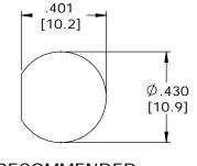
RECOMMENDED PANEL CUT-OUT TOLERANCE: ±.003
