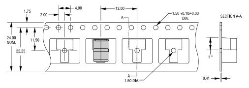
TOLERANCES: ±0.13 UNLESS OTHERWISE SPECIFIED **DIMENSIONS: MILLIMETERS**
