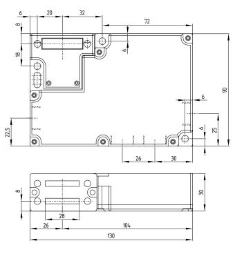
Solenoid interlock with prorective enclosure
