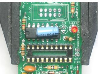
Next are the two capacitors, **C1** and **C2**. These provide some power supply filtering so that the USBtinyISP is less flakey. **C1** goes in the corner next to the USB connector. It is a non-polar ceramic capacitor so it can go in either way.
