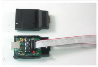
Plug in the two cables as shown, the red stripes on top and so that the cables don't bend over the plug (the case won't fit).
