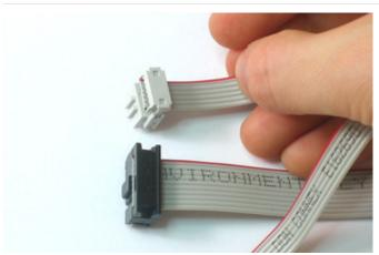
It's important that the key (the bump in the connector) and the red stripe line up. Match the image on the left, just poke the conductor in with a mm or two past the edge.
