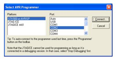
You should be able to communicate to your target, through the sofware. If you're having problems talking to the chip, check the power, whether a crystal or clock is necessary and that the ISP clock is not too fast! You can change the ISP clock in the Board tab of AVR studio:
