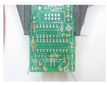
Now that you have a lot of practice with resistors, you can do the remaining 5 all at once. Place **R10** (10K pullup resistor), **R3**, **R5** and **R6** (1.5K resistors for the USB connection, LEDs and output buffer).
