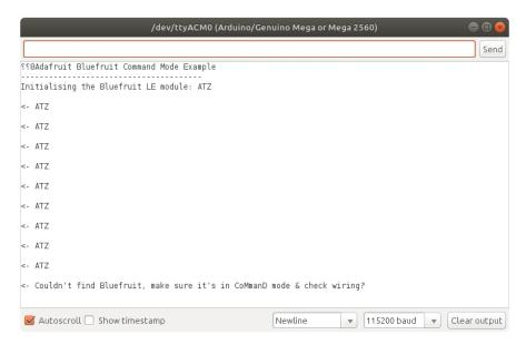
Then double check your wiring and make sure the slide switch is in the CMD position. If that all seems OK, you can also try power cycling the Bluefruit LE UART Friend. Simply remove the 5V wire for a sec and then reconnect it. Then try running the sketch again. Hopefully it'll start responding then.
