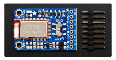
HW flow control (CTS+RTS) should always be used with the nRF51822. The UART peripheral block is designed in a way that more or less requires HW flow control for reliable UART communication, with a very small internal buffer and tight timing limitations due to the SoftDevice architecture (Nordic's proprietary Bluetooth Low Energy stack).
