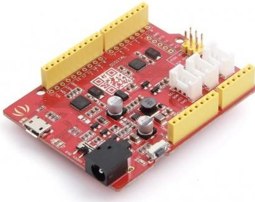
Seeeduino V4.2 is an Arduino-compatible board, which is based on ATmega328P MCU. There're so many Arduinos and Arduino-compatible boards in the world, and we think that Seeeduino V4.2 is one of the best Arduinos, Seeeduino V4.2 is much more stable, easy-to-use and even good looking.
