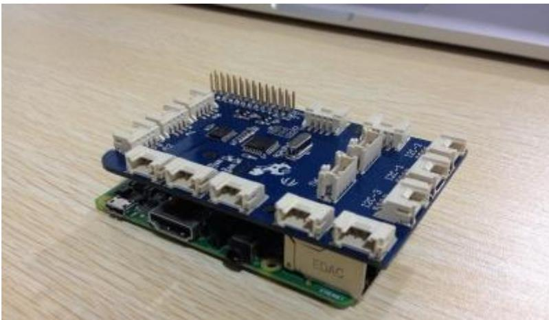
Ensure that the pins are properly aligned when stacking the GrovePi.
