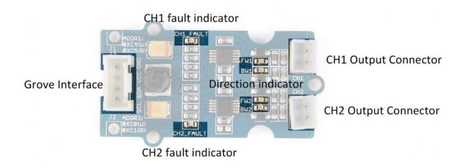
• **Grove Interface** - Grove products have a eco system and all have a same connector which can plug onto the <u>Base Shield</u>. Connect this module to the I<sup>2</sup>C port of Base Shield, and then it can work well with Arduino. However, you can also connect Grove - Mini I2C Motor Driver to Arduino without Base Shield by jumper wires.
