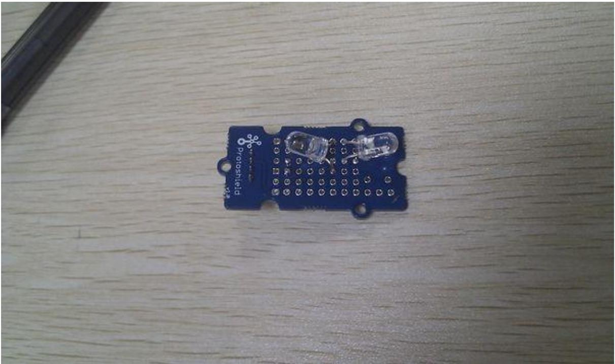
3. Connect the module to the Digital 8 of Grove - Basic Shield using the 4-pin grove cable.
