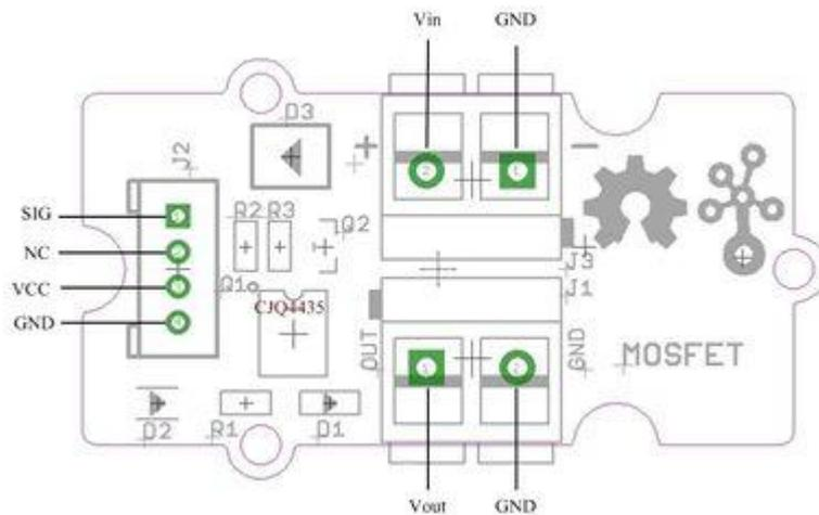
Vin: accepts 5V ~ 15V power of which current is less than 2A.
