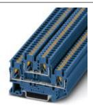
Double-level terminal block, connection method: Push-in connection, cross section: 0.14 mm² - 4 mm², AWG: 26 - 12, width: 5.2 mm, color: blue, mounting type: NS 35/7,5, NS 35/15
