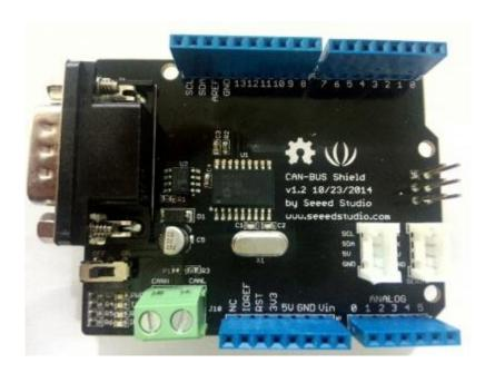
CAN-BUS is a common industrial bus because of its long travel distance, medium communication speed and high reliability. It is commonly found on modern machine tools and as an automotive diagnostic bus. This CAN-BUS Shield adopts MCP2515 CAN Bus controller with SPI interface and MCP2551 CAN transceiver to give your Arduino/Seeeduino CAN-BUS capibility. With an OBD-II converter cable added on and the OBD-II library imported, you are ready to build an onboard diagnostic device or data logger.
