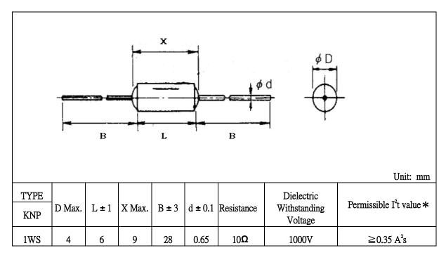
\* The exponential pulse waveform was used to determine the permissible  $I^2t$  value.
