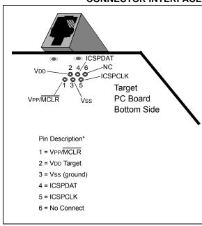
Another connector often found in use with the PICkit™ programmers is a standard 6-pin header with 0.1 inch spacing. Refer to Figure 22-2.
