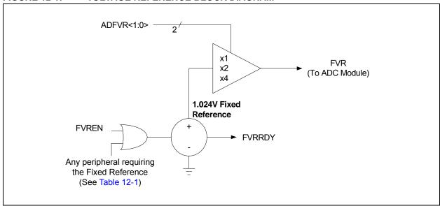
TABLE 12-1: PERIPHERALS REQUIRING THE FIXED VOLTAGE REFERENCE (FVR)
