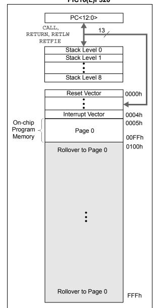
FIGURE 2-2: PROGRAM MEMORY MAP AND STACK FOR PIC10(L)F322
