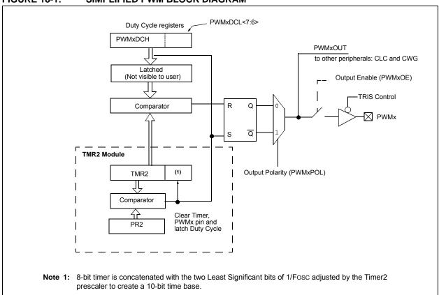
For a step-by-step procedure on how to set up this module for PWM operation, refer to Section 18.1.9 "Setup for PWM Operation using PWMx Pins".
