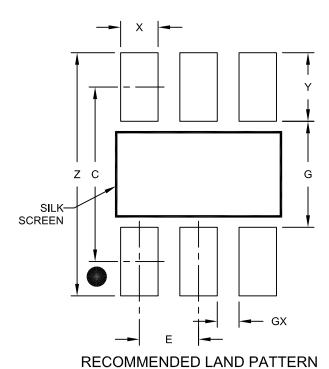
Units **MILLIMETERS Dimension Limits** MIN MOM MAX Contact Pitch 0.95 BSC Ε Contact Pad Spacing С 2.80 Contact Pad Width (X6) 0.60 Χ Contact Pad Length (X6) Υ 1.10 Distance Between Pads G 1.70 Distance Between Pads GX 0.35 Overall Width 3.90
