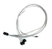
The Adaptec I-HDmSAS-4SATA-SB-.8M is an internal mini SAS HD x4 (SFF-8643) to (4) x1 Serial ATA (adapter based) fan-out cable with sideband signals. It measures .8 meters and is used for connecting a Series 7/7Q/7H/7He adapter to SATA disks, or a SAS/SATA backplane.
