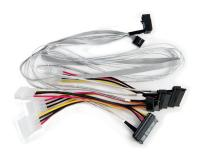
The Adaptec I-rA-HDmSAS-4SAS-SB-.8M is an internal right-angle mini SAS HD x4 (SFF-8643) (4) x1 Serial Attached SCSI (SFF-8482, adapter based) fan-out cable with sideband signals. It measures .8 meters and is used for connecting a Series 7/7Q/7H/7He adapter to SAS disks.
