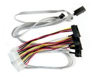
The Adaptec I-HDmSAS-4SAS-SB-.8M is an internal mini SAS HD x4 (SFF-8643) to (4) x1 Serial Attached SCSI (SFF-8482 adapter based) fan-out cable with sideband signals. It measures .8 meters and is used for connecting a Series 7/7Q/7H/7He adapter to SAS disks.
